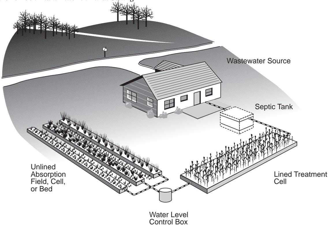
**Lined Treatment Cell.** The lined treatment cell with wetland plants provides essential wastewater treatment. The amount of treatment achieved through the treatment cell depends on the detention time (time required for flow through the cell), organic load, and treatment parameters such as oxygen and water temperature. Though significant treatment is provided by the lined treatment cell, effluent quality, especially for bacteria content, is not high enough to allow surface flow from the site.
